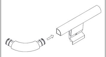
3. Insert corner casting into side rail as shown
