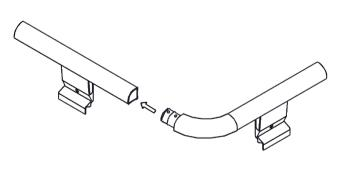
6. Insert the side rail assembly into the cross rail as shown
